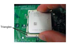
3. Align pin 1 of the CPU with pin 1 of the socket. Once aligned, <u>carefully</u> place the CPU into the socket. Do not drop the CPU on the socket, move the CPU horizontally or vertically or rub the CPU against the socket or against any pins of the socket, which may damage the CPU and/or the socket.
